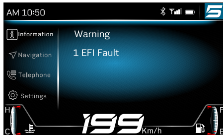
Example with fault.
